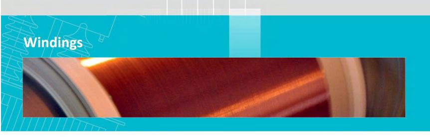
The low voltage windings are usually made by flat section electrolytic copper. CTC copper are used for transformers rated power up to 1000 kVA. Winding insulation are creating by craft or nomex. Cross section of the wires are calculating by special design softwares to reach higher level of cooling and lowest level of onload losses.
